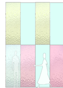
CLEAR AND REPILED COLOURED GLASS PATTERN TO DESIGN CLEAR VISION PANELS CRISTE FOR PRIVACY COLOUR BACKED GLASS TO 15 PLANTER EDGES
